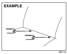
2) Place the child restraint in the rear seat, inserting the connecting bars through the slots in the seat cushion or the slots in the seatback bottom.
